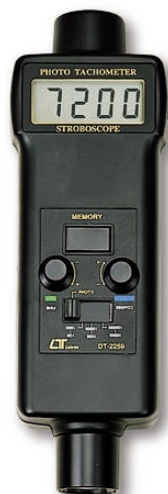
TACHOMETER/STROBOSCOPE Model : DT-2259 * Tachometer combines Stroboscope. 2 in 1. * Photo Tach. : 5 to 99,999 RPM. * Stroboscope : 100 to 100,000 FPM/RPM. * 4 x 1.5 V, AA(UM-3) battery power. * Size : 215 x 65 x 38 mm.
